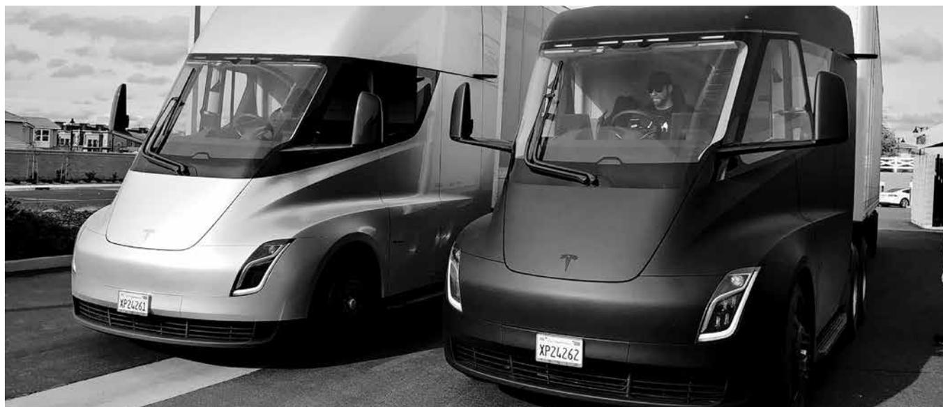
*Two Tesla Semi prototypes in 2018. Their specifications claim a 300-mile range for the base model, and acceleration of zero to sixty miles per hour in twenty seconds, fully loaded. The base price is \$150,000. Production of “limited volumes” is expected to begin in 2020. According to Equipment World, “electric trucks will require less maintenance since they feature fewer moving parts and require less fluid changes.”*
